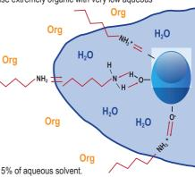
The mobile phase must contain a high proportion of organic solvent and at least 5% of aqueous solvent. The organic solvent is a weak solvent, while the aqueous solvent is stronger. For the utilisation on LC/MS, prefer volatile buffers.
